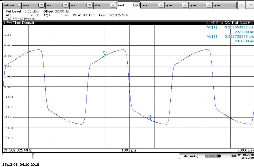
Figure 2 - Modulation with a repeated '00FF' word, Mod 2 = 0dB, Mod 1 = 2dB.
